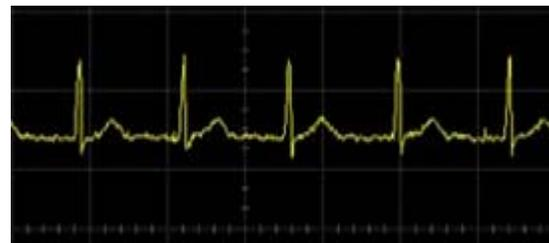
Fig. 14: Normal ECG waveform recorded from the prototype.
