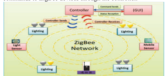
Figure 5 Structure of Sending and receiving packets The controller receives wireless signals from lighting
