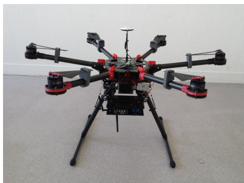
Fig. 3. Embedded sounder on a drone.
