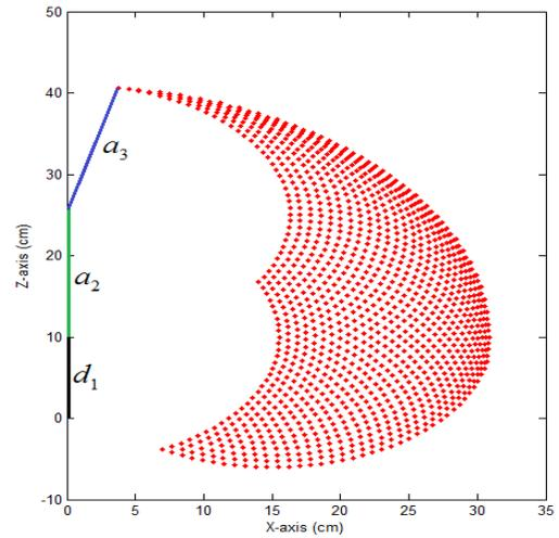
Figure 4: workspace of the arm at  $\theta_1=0$  in X-Z plane.
