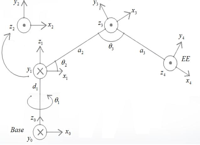
Figure 3: Reference coordination system for robot arm.
