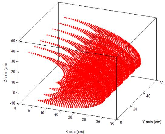
Figure 5: workspace of the arm at  $\theta_1=0$  along the path.
