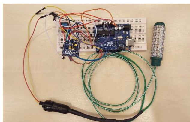
Fig. 3 Prototype of the wireless sensor node for soil moisture and air temperature measurement
