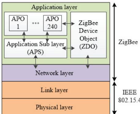
Fig. 1. ZigBee standard architecture of functional layers and protocol stack [4]
