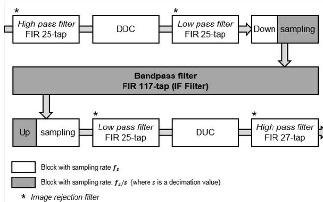
Fig. 1. Digital IF filter using Filter bank
