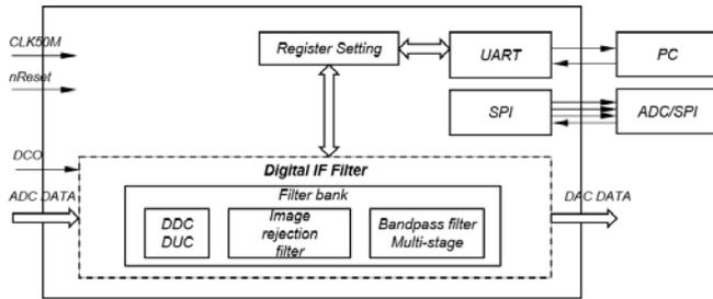
Fig. 3. Block diagram of digital IF filter.
