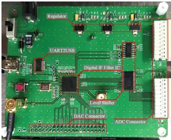
Fig. 4. Test board of proposed digital IF filter.
