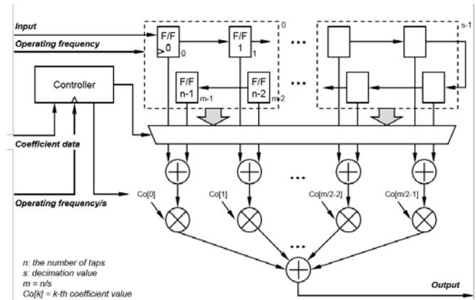
Fig. 2. Digital bandpass filter with Multi stage in Filter bank
