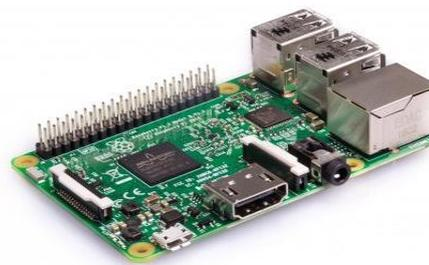
Fig. 2. Raspberry Pi 3 Model B as a single-board computer with wireless LAN and Bluetooth connectivity
