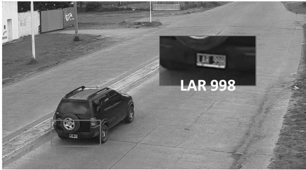
Fig. 1. A LPR detection case
