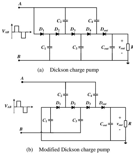
Fig. 2. Conventional and modified Dickson charge pump voltage multiplier circuits
