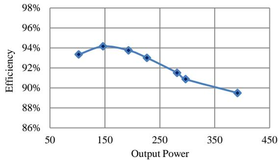
Fig. 13. Efficiency curve of the proposed converter
