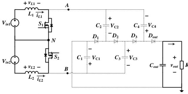
Fig. 5. Proposed converter operation in mode-I
