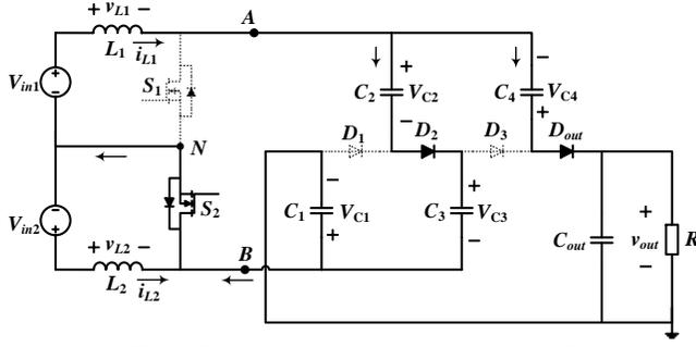
Fig. 6. Proposed converter operation in mode-II
