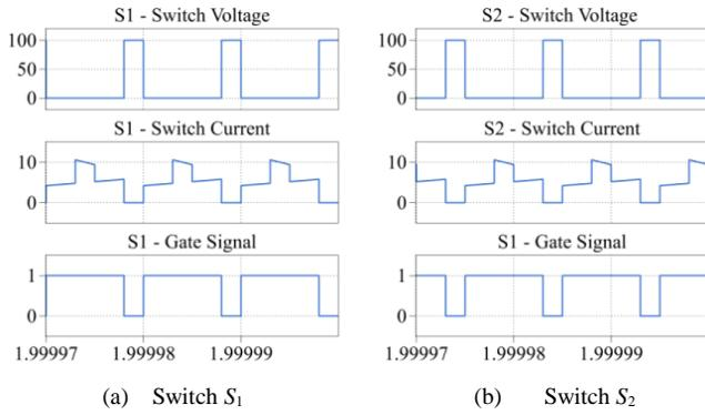
Fig. 10. Switch voltage, current and gate signal waveforms
