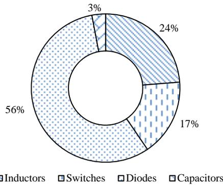
Fig. 12. Percentage distribution of losses in system components
