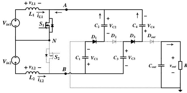
Fig. 7. Proposed converter operation in mode-III
