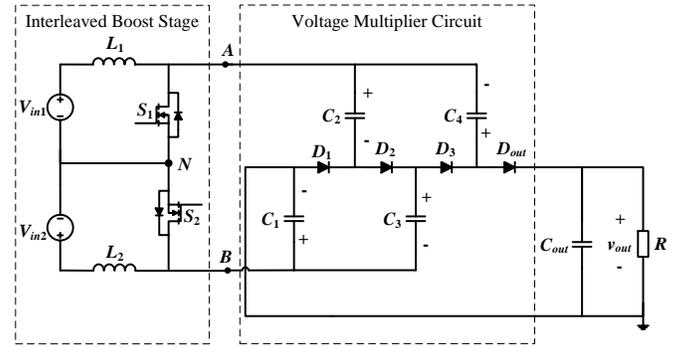
Fig. 3. Proposed high-voltage-gain dc-dc converter
