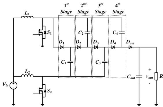
Fig. 1. High-voltage-gain dc-dc converter proposed in [19]
