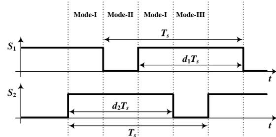
Fig. 4. Input boost converter switching signals for the proposed converter
