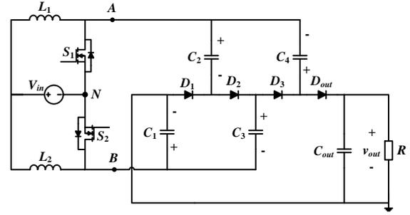
Fig. 8. Proposed converter with single input source
