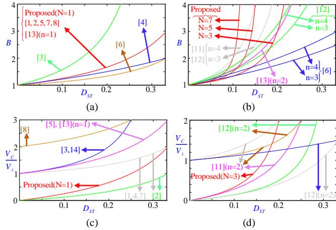
Fig. 6. Comparison of the proposed and conventional inverters; (a) in terms of boost factor ( $N = 1$ ); (b) in terms of boost factor ( $N > 1$ ); (c) in terms of capacitors voltages stresses ( $N = 1$ ); (d) in terms of capacitors voltages stresses ( $N > 1$ ).
