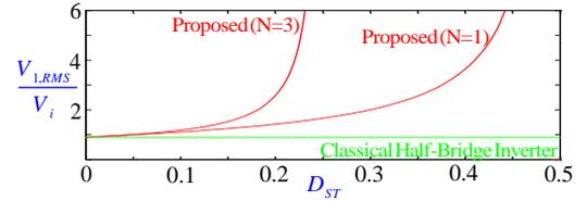
Fig. 7. Comparison between the proposed and classical half-bridge inverters as regard to the RMS value of fundamental harmonic of the output voltage.
