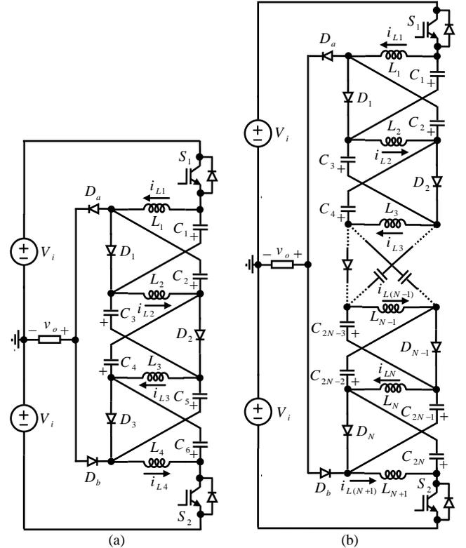
Fig. 5. Extension of the proposed topology; (a) with three Z-networks; (b) with  $N$  Z-networks.
