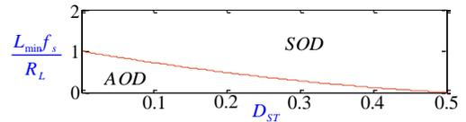
Fig. 4. Normalized  $L_{\min}$  versus  $D_{ST}$  at the SOD/AOD boundary.
