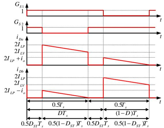
Fig. 3. The currents through diodes  $D_a$  and  $D_b$  in boundary operation between SOD and AOD.
