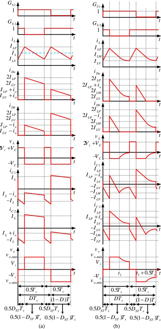
Fig. 2. The voltage and current waveforms of the proposed topology; (a) in SOD; (b) in AOD.
