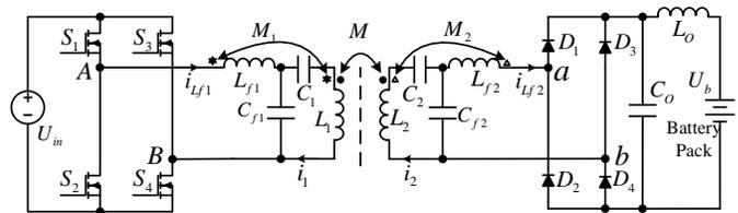
Fig. 1. Studied integrated LCC compensation topology.
