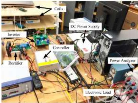
Fig. 7. Experimental setup for a WPT system.
