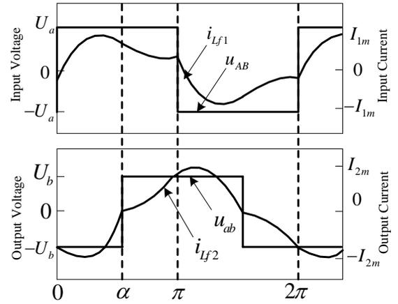
Fig. 3. Theoretical waveforms of CCM.
