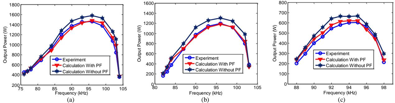
Fig. 14. Experimental and calculated output power of the WPT system at different frequencies. (a)  $X=0\text{mm}$ ,  $Y=0\text{mm}$ . (b)  $X=200\text{mm}$ ,  $Y=0\text{mm}$ . (c)  $X=0\text{mm}$ ,  $Y=150\text{mm}$ .
