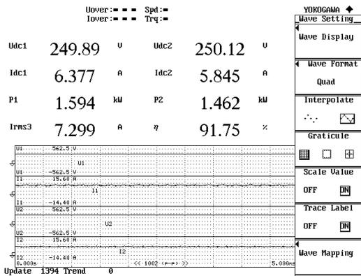
Fig. 9. Capture of power analyzer @96kHz with no misalignment.
