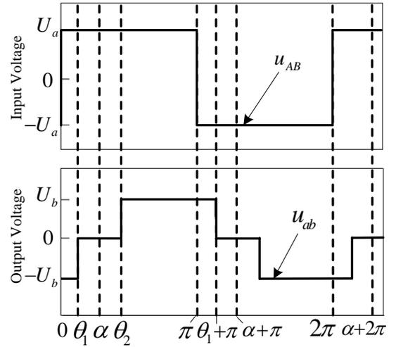
Fig. 5. Equivalent voltage waveforms of DCM.
