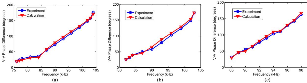
Fig. 12. Experimental and calculated phase differences between input and output voltages of the WPT system at different frequencies. (a) X=0mm, Y=0mm. (b) X=200mm, Y=0mm. (c) X=0mm, Y=150mm.
