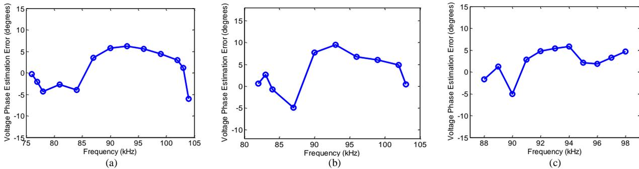
Fig. 13. Estimation errors between experimental and calculated results of input and output voltage phase difference at various frequencies. (a)  $X=0\text{mm}$ ,  $Y=0\text{mm}$ . (b)  $X=200\text{mm}$ ,  $Y=0\text{mm}$ . (c)  $X=0\text{mm}$ ,  $Y=150\text{mm}$ .
