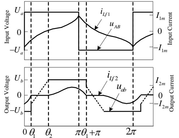
Fig. 4. Theoretical waveforms of DCM.
