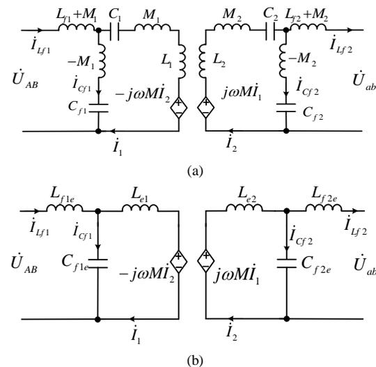
Fig. 2. Equivalent circuits. (a) Decoupled circuit model. (b) Simplified equivalent circuit model.
