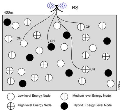
Fig. 6: Four energy level nodes with their cluster heads.
