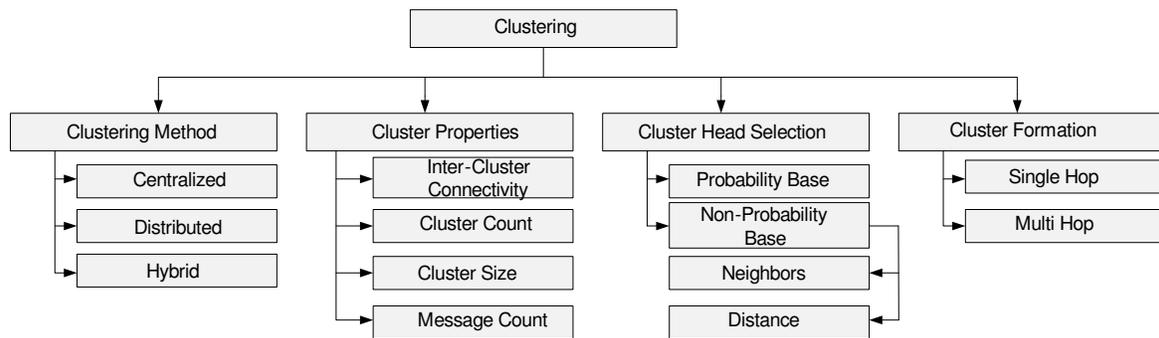
Fig. 3: Clustering in WSNs can be achieved by considering clustering method, clustering properties, cluster head selection procedure, and cluster formation
