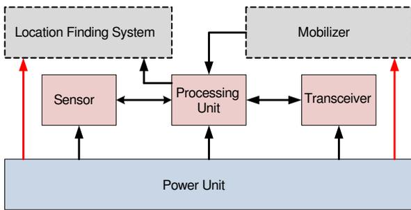
Fig. 1: The architecture of the sensor node consists of power unit, sensor, processing unit, transceiver, location finding system, and mobilizer
