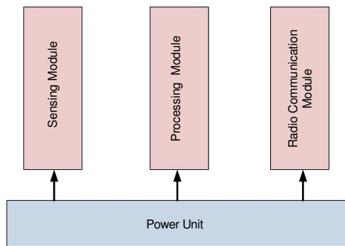
Fig. 4: Sensor node with three main modules.
