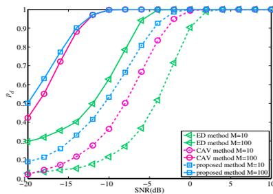
Fig. 5. Sensing performance of the proposed algorithm under different  $M$
