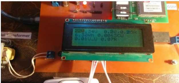
Fig. 14. Proposed Meter Readings for 60W Load
