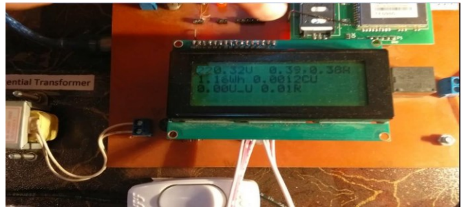
Fig. 12. Proposed Meter Readings for 120W Load
