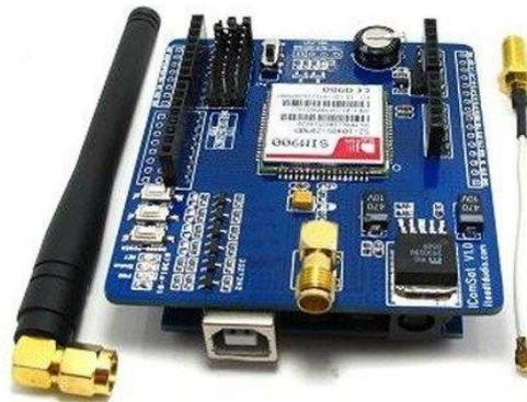
**Figure 2.** The GSM SIM900A module to communicate with Arduino board.
