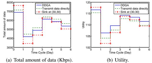
Fig. 6. Total amount of data for the entire network in each day and corresponding utility obtained by DDGA, direct transmission scheme and optimal data gathering for an RSN with a static sink node at (30, 30), respectively.
